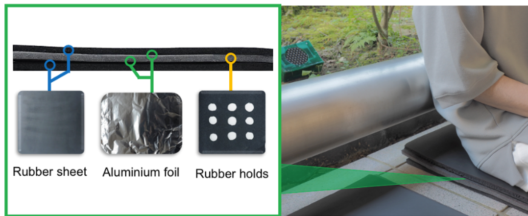
Figure4.4 Hardware design in specific scenarios; the capacitive sensor
