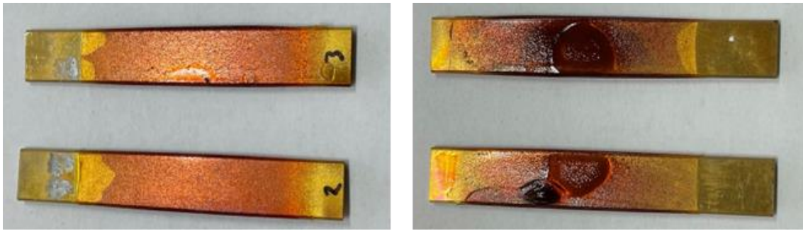
Fig 5-14. Appearance of PAA varnish electrostatic spray-applied test piece (110°C)
