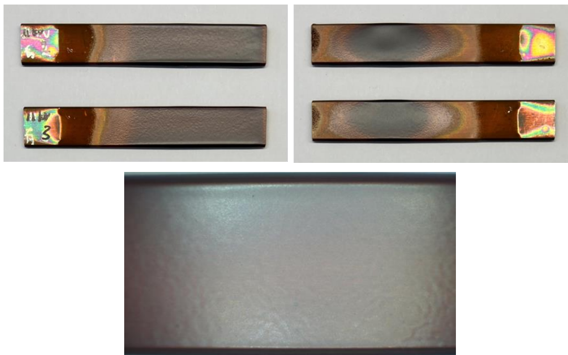
Fig 5-20. Appearance of electrostatic spray-applied test piece Run3 (Alu C805)
