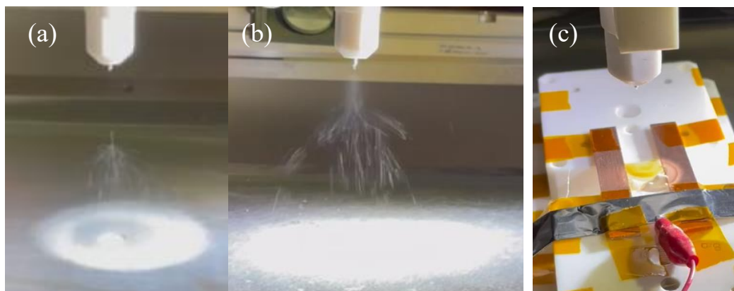
Fig 5-8. Spray shapes of (a)Ramified-jet , (b)random, (c)spider threa-like
