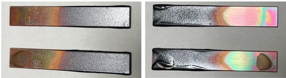
Fig 5-15. Appearance of PAA varnish + MgO electrostatic spray-applied test piece (110°C)
