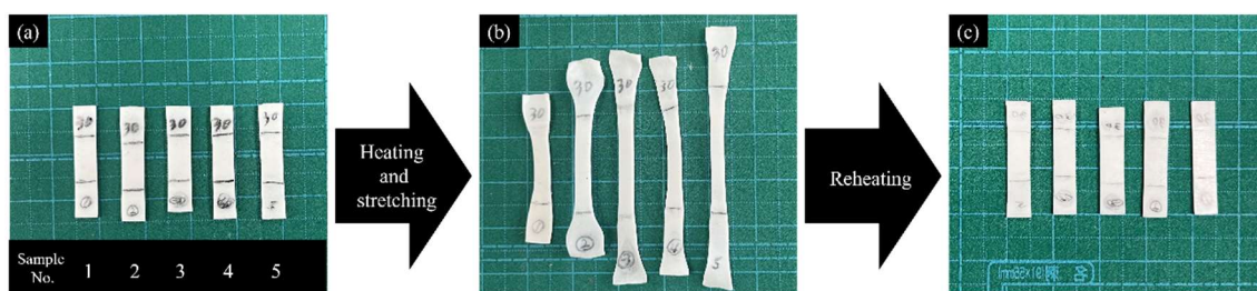
Figure 8.14. Image of heat contraction behavior of V35-RY40-PE30.
