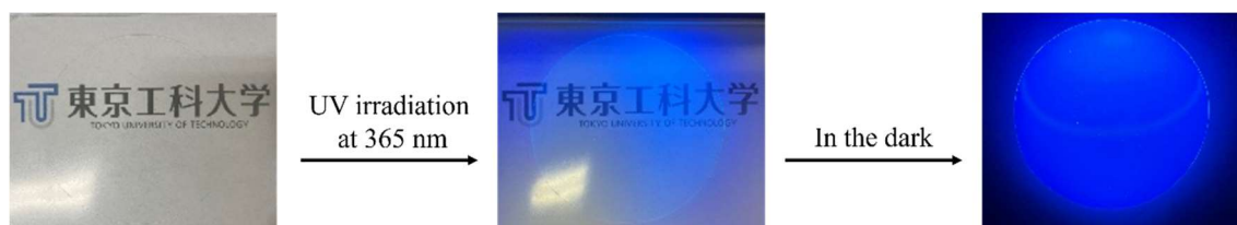
Figure 6.21. Image of Poly(DPEPM/MMA/BA) film (Run8) emit by UV irradiation at 365 nm.
