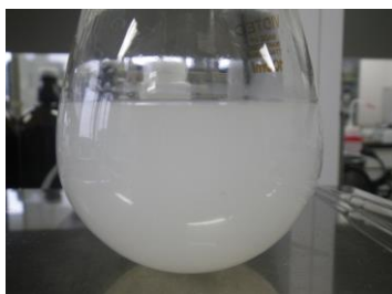
Figure 2-4. Photo of suspension of PAA particles obtained by the addition of THF and tripropylamine (run3 in Table 2-2).
