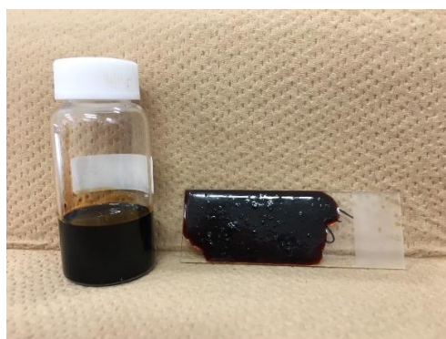
Figure 7-4. Photos of the mixed sample of glycol-lignin, epoxy resin, and DBU-PhR before (left) and after (right) thermal treatment.
