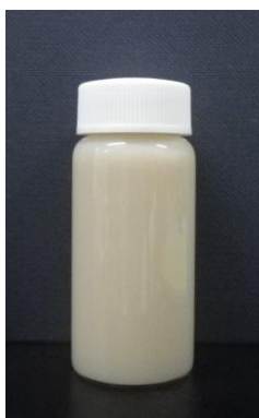
Figure 5-17. Image of nanoparticle dispersion mixture of PI(BTDA/AHPP)-DAA and Alumina.
