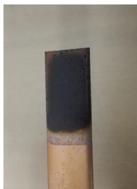
Figure 5-19. Image of the cathode after electrodeposition coating by PI(BTDA/AHPP)-DAA/Alumina composite and annealing at 200 °C for 30 min.
