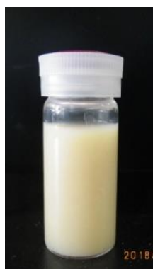
Figure 5-7. Image of nanoparticle dispersion solution containing PI(BTDA/AHPP)-DAA (run 4 in Table 5-1).
